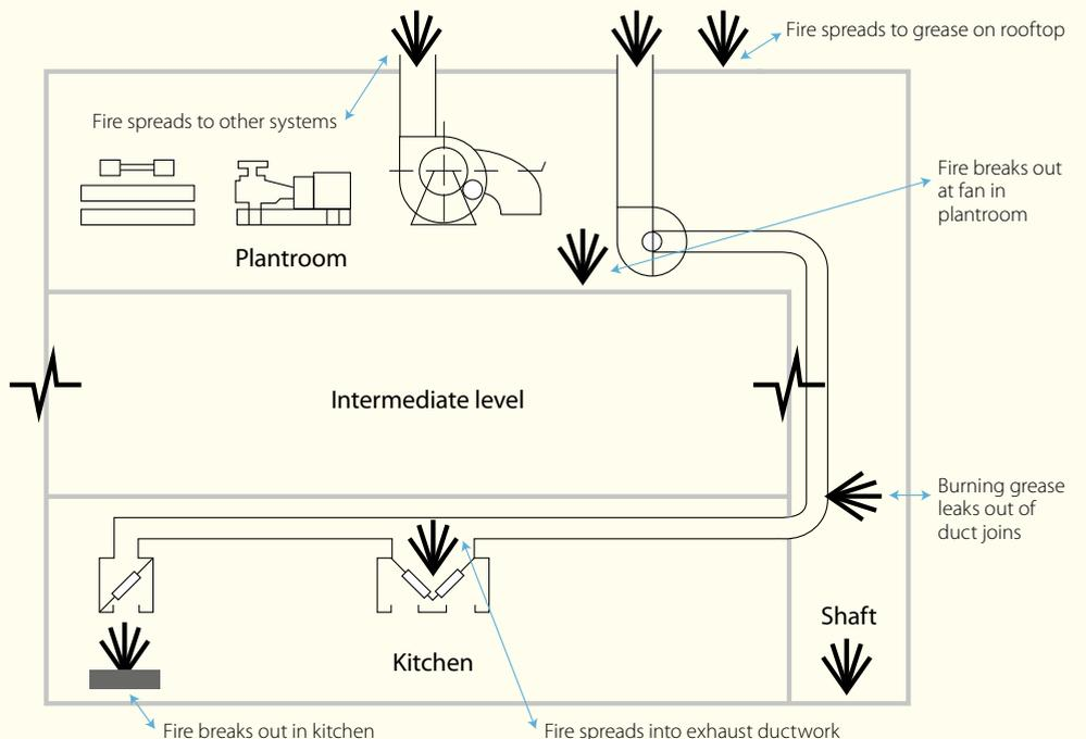
Fig 1: Fire in kitchen spreading into duct and then fire in duct spreading/breaking-out to another area.
