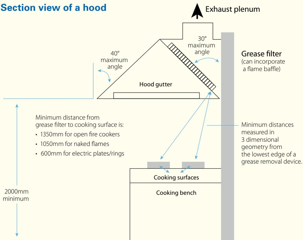
Fig 2: Minimum filter separation to cooking surface.
