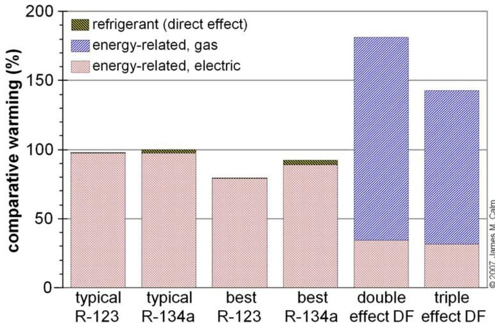
Figure 3. Comparative Global Warming Impacts for Typical and Best Available R-123, R-134a, and Direct-Fired, Water/Lithium Bromide Absorption Chillers (including condensing water pump and cooling tower energy use all normalized to typical R-134a chiller impacts)
