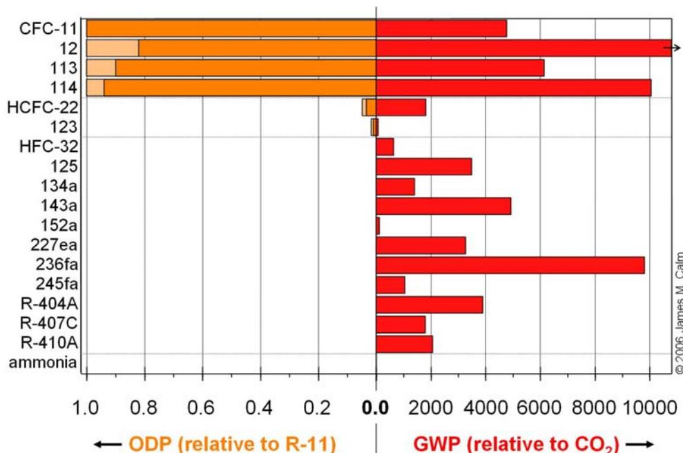
Figure 2. Ozone Depletion Potential (ODP) Contrasted to Global Warming Potential (GWP) for Key Refrigerants (light and dark orange shading indicate semi-empirical and modeled ODPs, respectively). CFCs generally have high ODP and GWP. HCFCs generally have much lower ODP and GWP. HFCs offer near-zero ODP, but some have very high GWPs.
